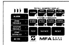
MFA6000-Series Keypad (behind front door) with LED indicators at left, and mini-sounder and numeric display just above.
